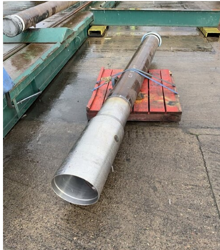
Helix with 10-3/4" pup welded on
